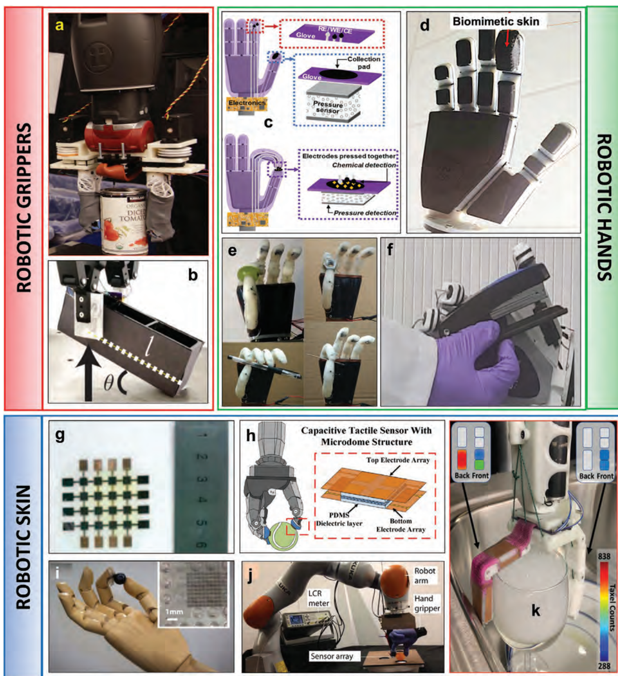
Figure 10. Flexible capacitive pressure sensor for robotics applications. a) Soft robotic puncture resistant gripper holding an object for material detection and sorting. Both fingers of the soft robotic gripper consist of flexible capacitive and strain sensors. Reproduced with permission. [163] Copyright 2019, IEEE. b) Soft robotic gripper; capacitive pressure sensors on the fingers have bumps to measure normal and shear pressure. Reproduced with permission. [165] Copyright 2020, IEEE. c) Schematics of robotic glove with capacitive pressure and chemical sensors designed for monitoring hazardous materials. Reproduced with permission. [166] Copyright 2019, RSC. d) 3D-printed robotic hand with biomimetic tactile sensor stack on index finger. Reproduced with permission. [167] Copyright 2019, Wiley. e) Soft robotic hand with integrated capacitive pressure sensors holding different materials. Reproduced with permission. [168] Copyright 2018, IOP Science. f) 3D-printed robotic hand with soft flexible capacitive pressure sensors on each finger holding a stapler. Reproduced with permission. [169] Copyright 2020, Wiley. g) Flexible capacitive sensory robotic skin utilized for tactile sensing. Reproduced with permission. [170] Copyright 2016, IEEE. h) Capacitive pressure sensor array which is fabricated using simple micromachining process has micro-dome structure. Reproduced with permission. [174] Copyright 2019, IEEE. i) Robotic hand holding the fabricated flexible capacitive robotic skin and inset shows close-up view of the micro-bumps and electrodes. j) Robotic skin mounted on commercially available robotic gripper is used for tactile sensing by capacitance change which is monitored using LCR meter. (i,j)—Reproduced with permission. [110] Copyright 2018, AAAS. k) The soft robotic gripper composed of flexible and stretchable robotic skin with capacitive pressure sensors holding a wet and soft object. Reproduced with permission. [175] Copyright 2020, IEEE.
